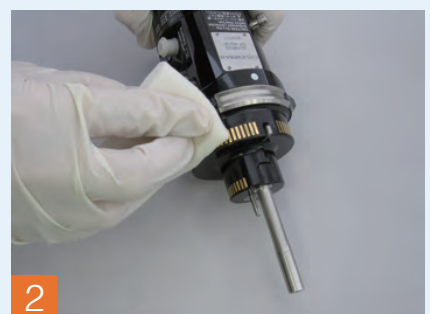
2 Wipe the electrical contacts and leave them to dry naturally.
