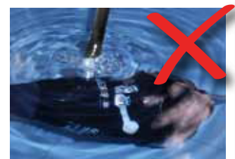
Bubbling during leakage test
