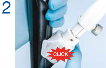
Secure the needle on the scope by pushing the bronchoscope adapter (connecting slider) to the "lock position" until it clicks.
